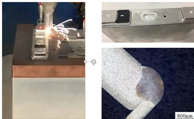
Figure 14. Photographs of Al lid-to-case welding. The left image shows a frame from a video of the welding process, the top-right image shows a finished cell, and the bottom-right images shows a magnified view of the weld cross-section.
