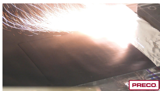
Figure 16. Photograph of remote cutting of coated Al foil using a 1.2 kW single-mode fiber laser.
