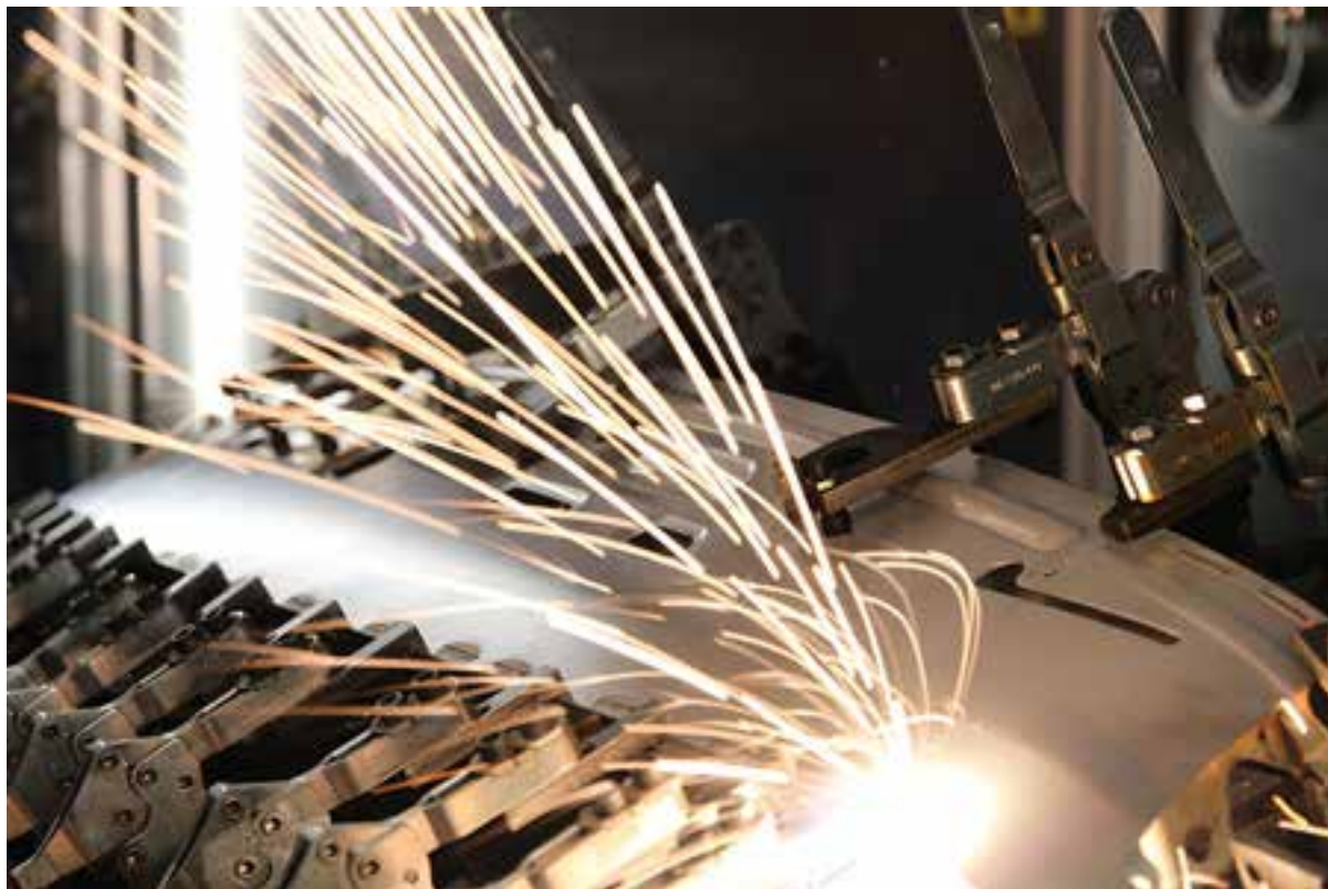
FIGURE 3. A Rofin scanner-based fiber laser welds automotive parts. (Courtesy of Rofin-Sinar)
