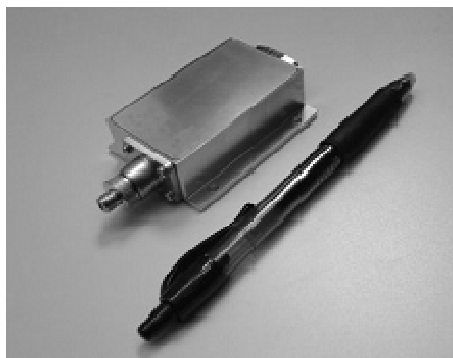
Figure 2. (Left) Photograph of a fiber-coupled module next to a common ink pen to emphasize its relative size. The unit weights ~500 grams. (Right) Module brightness can be scaled in three independent ways. Coupling to smaller fiber is achieved through improvements in optical alignment and diode emitter brightness.
