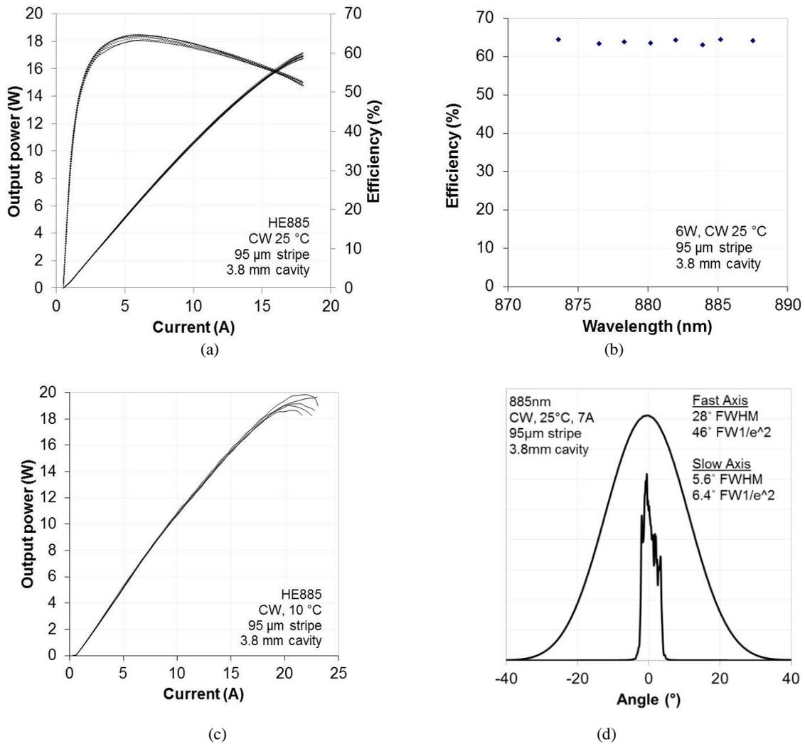
**Figure 2:** HE 88x nm lasers of 95μm stripe width and 3.8mm cavity length (a) typical power and efficiency at CW 25°C (b) efficiency versus wavelength at 6W 25°C (c) CW tested to rollover at 10°C (d) typical far field at 7A
