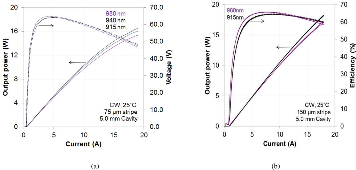
**Figure 4:** Typical continuous wave (CW) optical power and wall-plug efficiency versus drive current for 5.0 mm long 915/940/980 nm devices operating at 25°C (test station), with (a) 75  $\mu\text{m}$  wide stripe, (b) 150  $\mu\text{m}$  wide stripe
