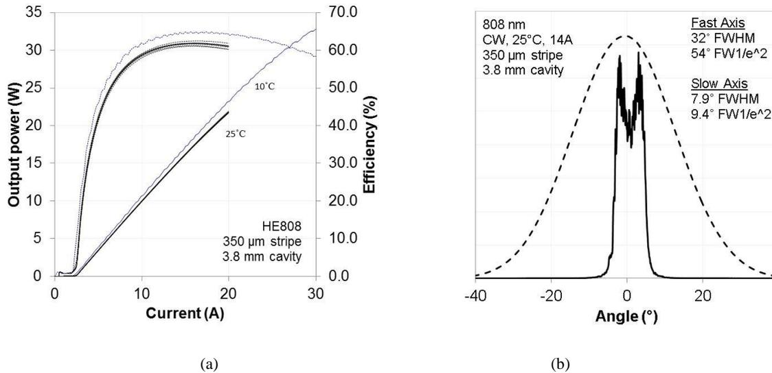
**Figure 1:** Performance of 15W 808 nm chip of 350  $\mu$ m wide stripe and 3.8 mm long laser cavity (a) power and efficiency at 25  $^{\circ}$ C and 10  $^{\circ}$ C (b) fast-axis and slow-axis far field at 14 A (15 W).
