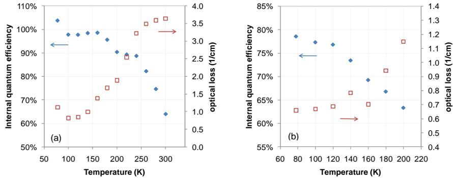
**Fig. 2:** Internal quantum efficiency ( $\eta_i$ ) and optical loss ( $\alpha_i$ ) as a function of temperature for (a) control design and (b) experimental design, retrieved from cutback experiments.
