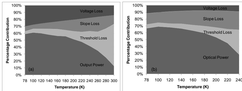
**Fig. 1:** Temperature dependence of main terms limiting efficiency for (a) the control design and (b) the experimental design with 1.5 mm cavity length. Measured at an injection current of 2 A.
