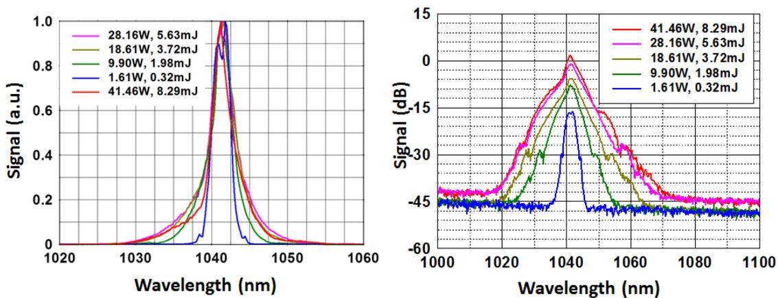
Figure 16. Pulse spectrum on a linear scale (left) and a log scale (right) vs. pulse energy. 8.29 mJ corresponds to a peak power of 640 kW.
