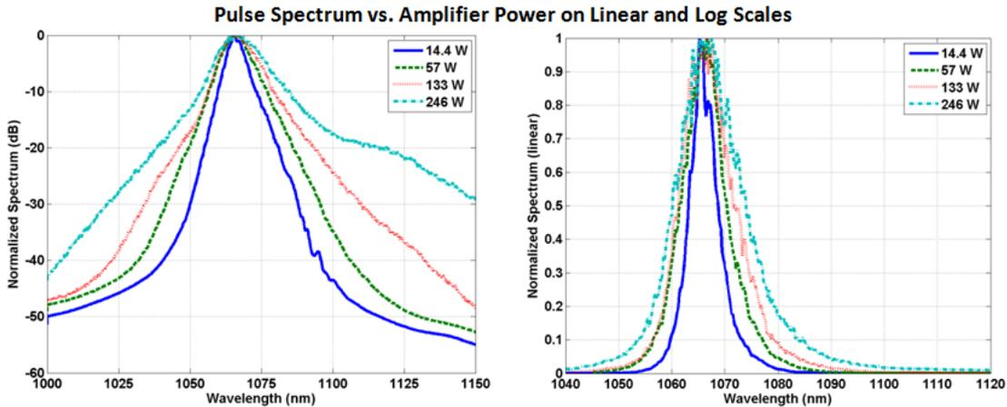
Figure 7. Pulse spectrum vs. amplifier in-core signal output power. The large bandwidth of the MOPA-M results in significant spectral broadening in the final amplification stage. The pulse energy associated with each average power curve is: 0.07mJ (14 W), 0.28 (57 W), 0.67 (133 W) and 1.23 mJ (246 W).
