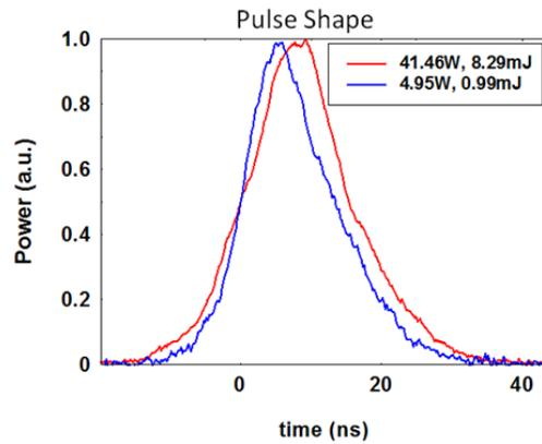
Figure 15. Pulse temporal shape at 0.99 and 8.29 mJ. The smooth spectral shape does not change significantly even at amplification to pulse energies up to 8X the saturation energy.
