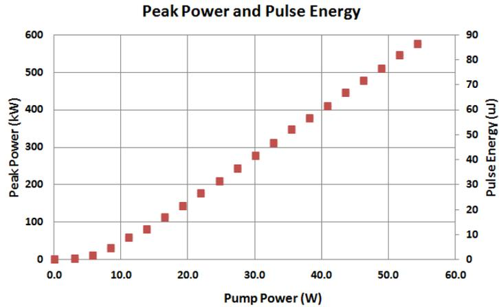
Figure 9. Pulse energy and peak power as a function of pump power.
