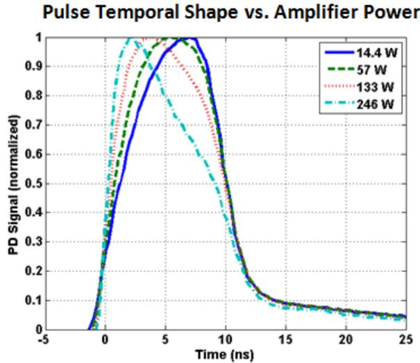
Figure 6. Pulse temporal shape vs. amplifier in-core signal output power. Gain saturation steepens the leading edge of the pulse as the power increases.
