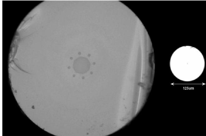
Figure 2. 55  $\mu\text{m}$  core 3C fiber with 8 side cores. A standard 6/125  $\mu\text{m}$  fiber is shown for reference.
