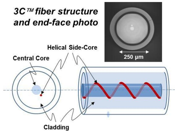
Figure 1. 3C fiber structure
