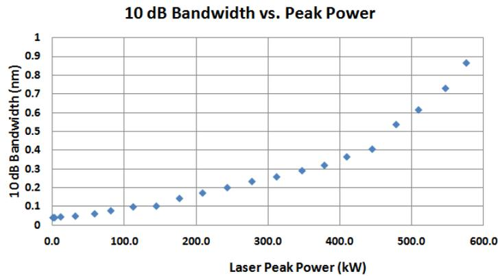
Figure 12. Pulse spectrum 10 dB bandwidth versus peak power.
