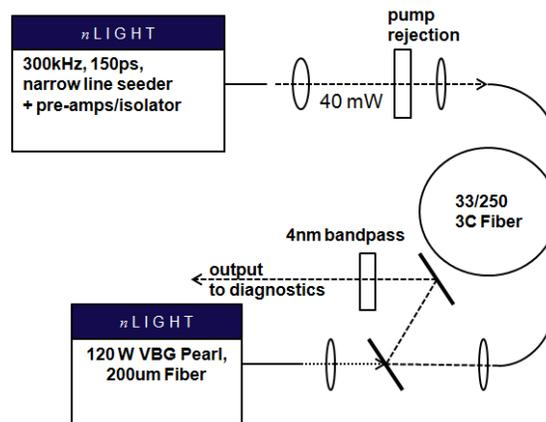
Figure 8. Experimental setup for characterizing 3C amplifier operation for high peak power sub-nanosecond pulses.
