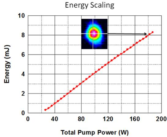
Figure 14. Pulse energy from the final stage 3C amplifier as a function of pump power. A single mode quality beam is maintained up to full power levels.
