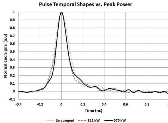
Figure 10. Pulse temporal shapes through an un-pumped amplifier (<math><0.07\text{ nJ}</math>), at 311 kW peak power (46.5 $\mu\text{J}</math>), and 575 kW peak power (86.5 $\mu\text{J}</math>). The pulse shape and duration remain largely unchanged. Pulses were measured with a 12GHz real-time oscilloscope and >15GHz bandwidth photodiode.$$
