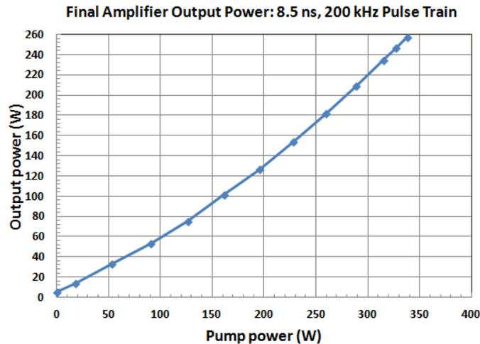
Figure 5. In-core signal output power versus 976 nm pump power.
