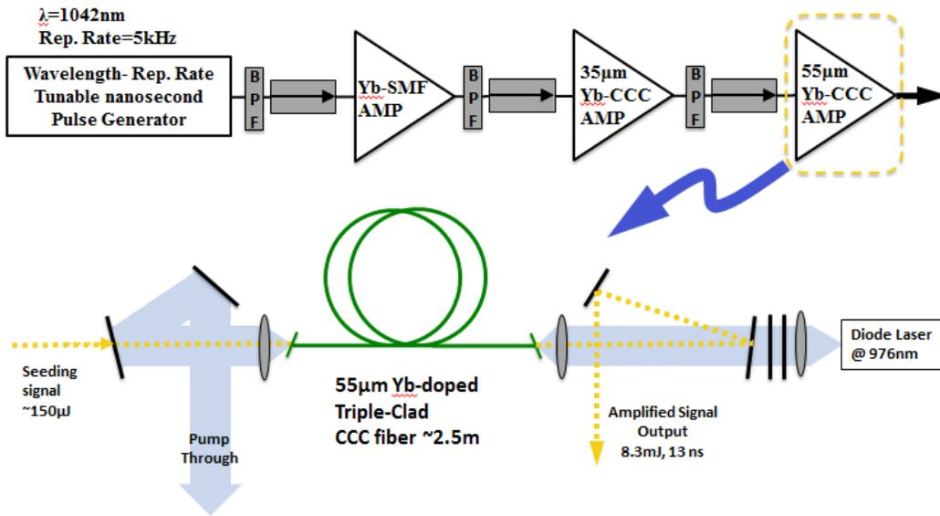
Figure 13. Diagram of experimental setup for pulse amplification in 55  $\mu\text{m}$  core 3C fiber amplifier.
