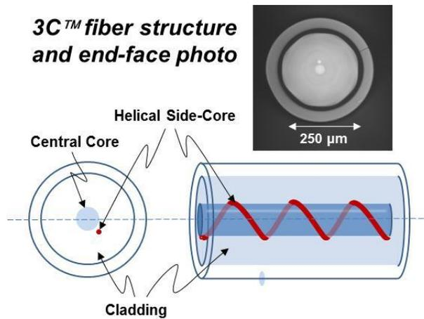
Figure 1. 3C fiber structure
