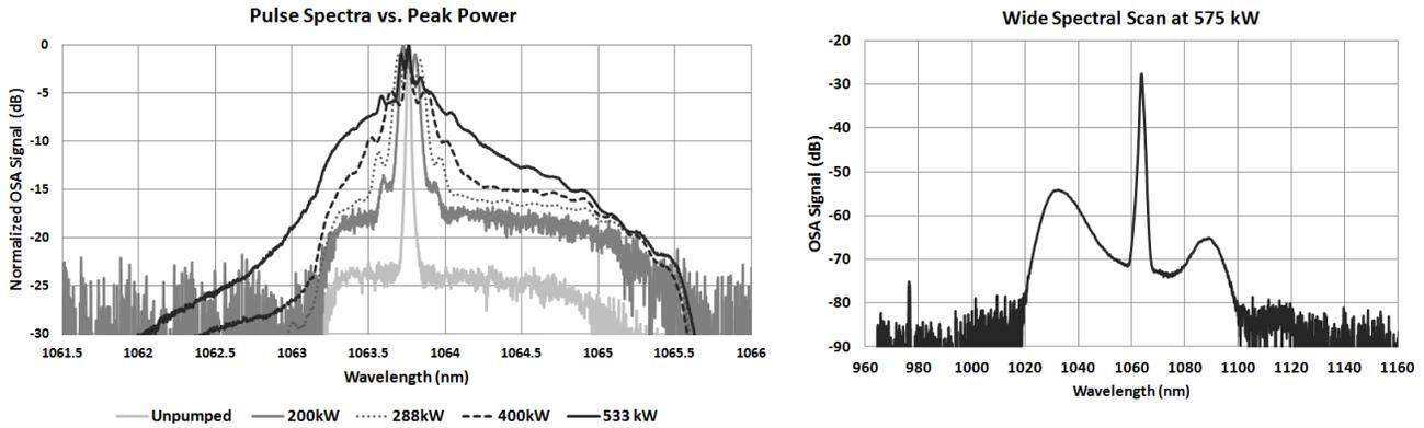
Figure 11. Left - amplified pulse spectrum as a function of the pulse peak power. Right - the spectrum of 575 kW peak power pulses over a wide spectral window.
