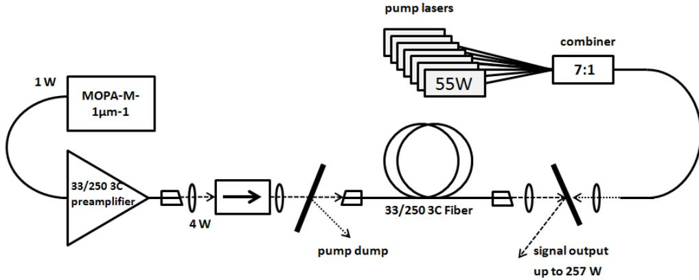
Figure 4. Diagram of experimental setup for high average power, large pulse energy 3C fiber amplifier characterization
