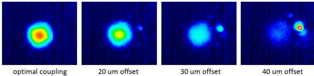
Figure 3. Output mode from 55  $\mu\text{m}$  core 3C fiber as the input is misaligned. There is no distortion of the central core mode even as the signal input misalignment becomes larger than the core radius of 25  $\mu\text{m}$ .
