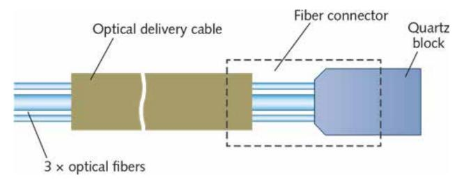
**FIGURE 2.** Three fiber core trifocal brazing optics enable different diameter fibers to pass through a single process cable to deliver spatially offset spots of different size to the brazing area.
