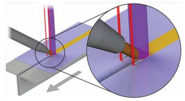
**FIGURE 1.** In trifocal brazing, two lead beams (red) clean and pre-heat the steel edge surfaces to promote wetting. The trailing beam (purple) melts the Cu/Si wire to form a seamless brazed joint which, after painting, can be invisible to the naked eye.
