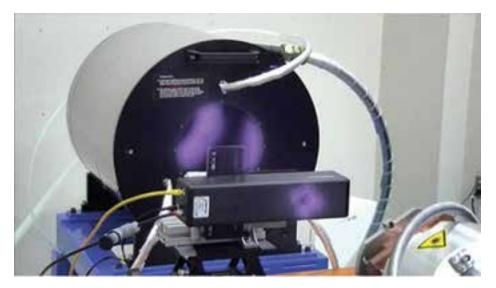
**FIGURE 3.** The beam power and profile of a 100 kW fiber-laser beam are measured at the same time via the combination of a calorimeter-based power sensor and Rayleigh-scattering beam profiler. (Courtesy of Ophir Photonics)
