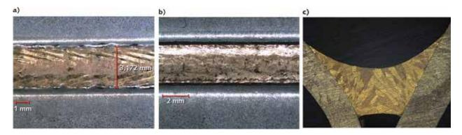
**FIGURE 3.** A comparison of single-spot (a) and trifocal (b) brazed seams that join steel with CuSi wire. An improved finish and suppression of edge roughness is evident in the trifocal brazing example. A cross-section (c) highlights the joint uniformity and quality obtainable with trifocal brazing.
