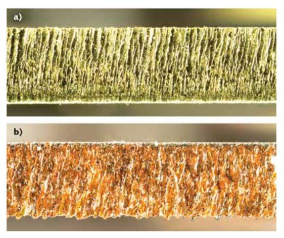
**FIGURE 6.** Immunity from back-reflections enable cutting of highly reflective metals that were problematic for first some-generation fiber lasers. Cross-section views show cuts created by a Coherent Highlight FL laser through 1.25-mm-thick brass (a) and 1.2 mm copper (b). (Courtesy of Coherent)
