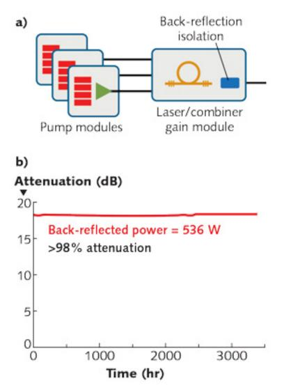
**FIGURE 4.** The nLIGHT alta design incorporates a back-reflection isolator between the laser and delivery fiber (a). A continuous laser-stability stress test with greater than 500 W directed back into the laser for thousands of hours shows no indication of unstable operation (b). (Courtesy of nLIGHT)
