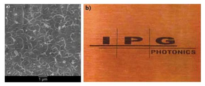
**FIGURE 5.** Example of the fine, nodular Cu surface structure (10,000X magnification) obtained using a sub-nanosecond NIR fiber laser (a). The textured Cu surface is perfectly black, making it an ideal absorber for subsequent laser processing (b).
