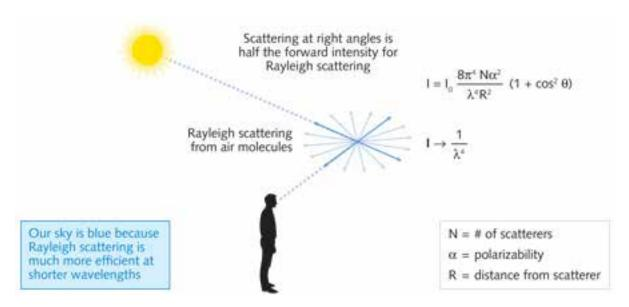
**FIGURE 1.** Rayleigh scattering of light from molecules in the air scales inversely with the fourth power of the wavelength.
