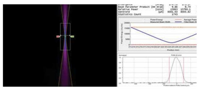
**FIGURE 2**. The operator screen for the BeamWatch Rayleigh-scattering-based beam profiler displays the beam along with its relevant parameters. (Courtesy of Ophir Photonics)
