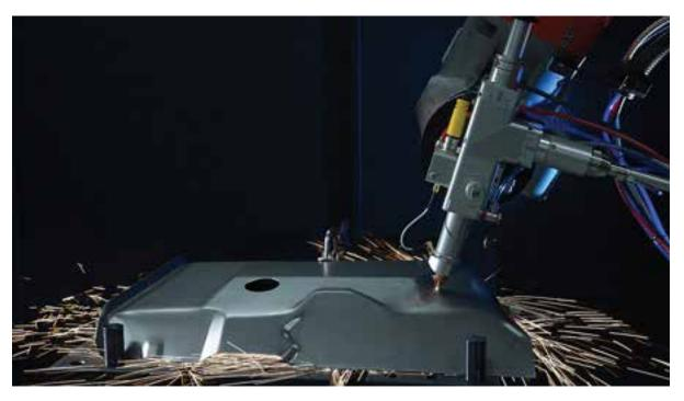
**FIGURE 5.** A Coherent Highlight FL fiber laser can be combined with robotics to enable high-speed 3D part cutting for industries such as white goods (washing machines, kitchen stoves, and so on). (Courtesy of Coherent)
